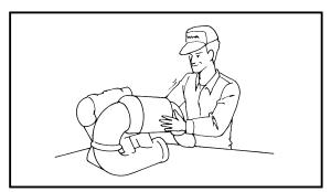
4. Install bearings with the manufacturer's markings on the side exposed to view and liberally oil the bearings.
