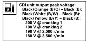
Cranking 1: unloaded Cranking 2: loaded
