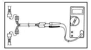
• When measuring the peak voltage, connect the peak voltage adaptor to the digital tester and switch the selector to the DC voltage mode.
